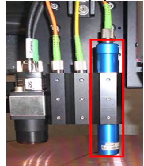
dedicated sensors: 2x CWL 600 µm (TTV setup)
